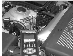
Access Diagnostic Trouble Codes (DTCs) to diagnose engine management problems.
